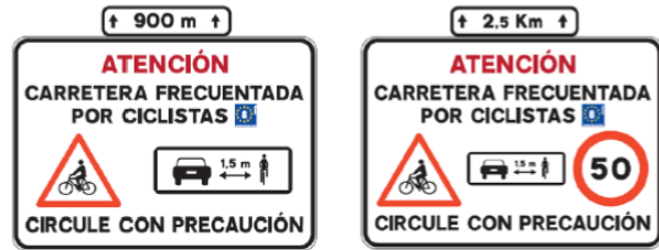
Mock-ups for warning signs for cars regarding the cycle route, in the Region of Murcia
