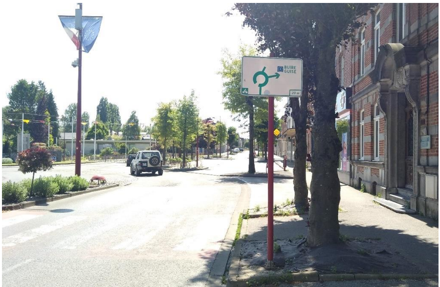
Example of an “Announce” sign in France, indicating a roundabout 20m away and which exit corresponds to EuroVelo 3
